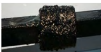
Untreated stainless steel level sensor removed from oil production tank after several weeks.
