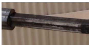
Treated stainless steel level sensor removed from oil production tank after 3 years.
